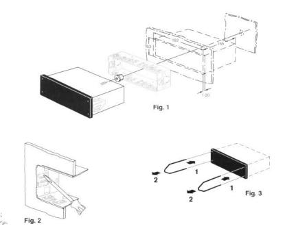
Removing the car radio
